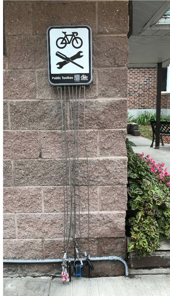
Figure D-12: A public toolbox/repair station in Westport at the Visitor Welcome Centre
