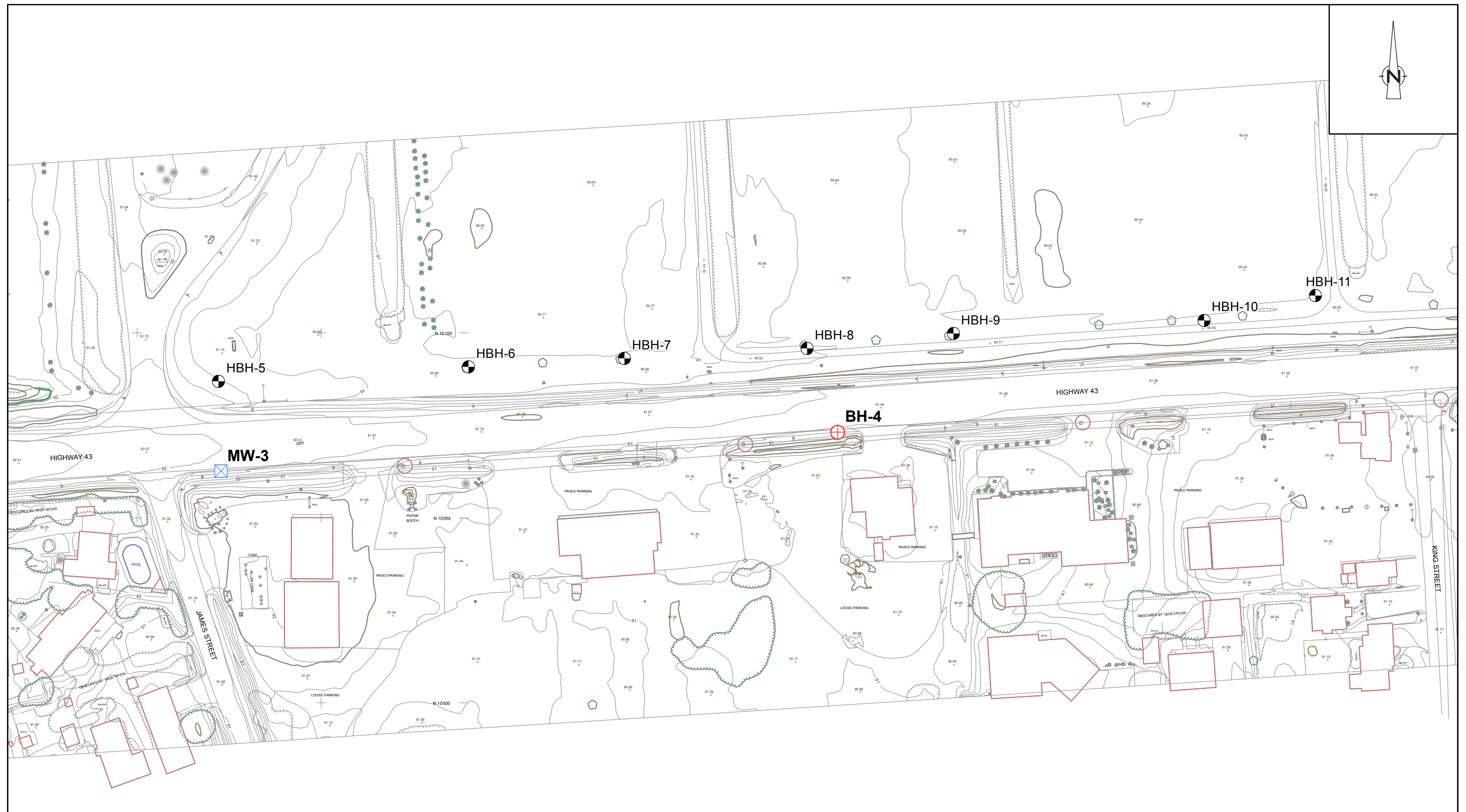
Figure 4: Corridor Borehole and Monitoring Well Location Plan - 2
