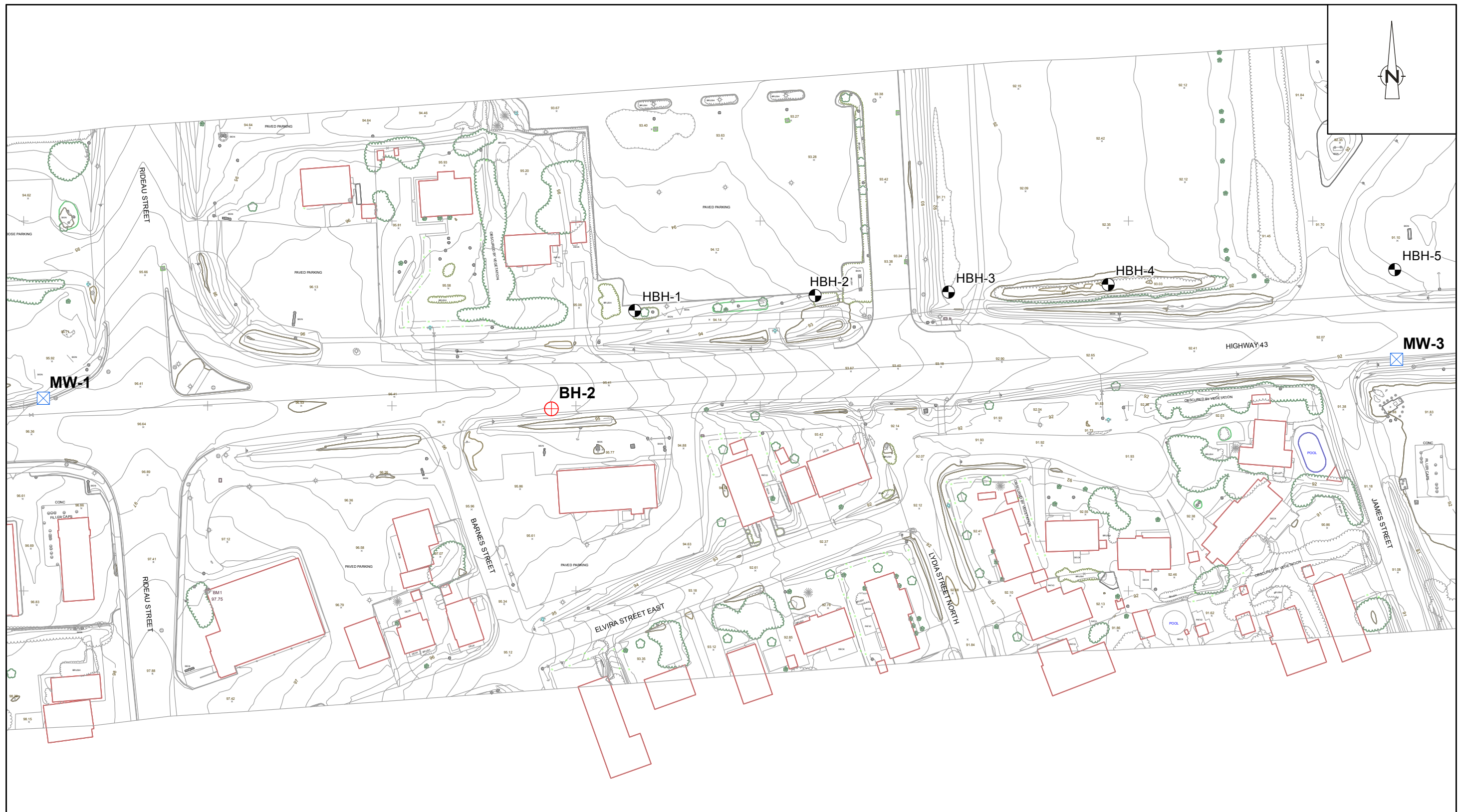
Figure 3: Corridor Borehole and Monitoring Well Location Plan - 1
