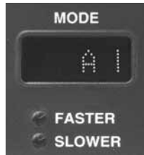
Figure 3.3e Initially, the letter “A” will indicate the Stationary Away Mode has been selected. The “A” will also appear when a target is acquired.
