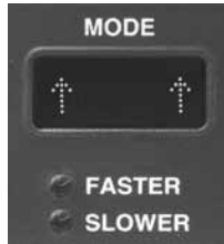
Figure 3.5b The MODE window when the unit is in Moving Mode Same Direction.
