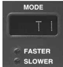
Figure 3.3c Initially the letter “T” will indicate the Stationary Towards Mode has been selected. The “T” will also appear when a target is acquired.
