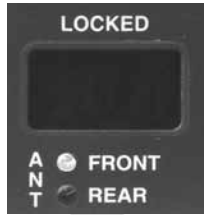
Figure 4.2c The FRONT and REAR antenna lights.
