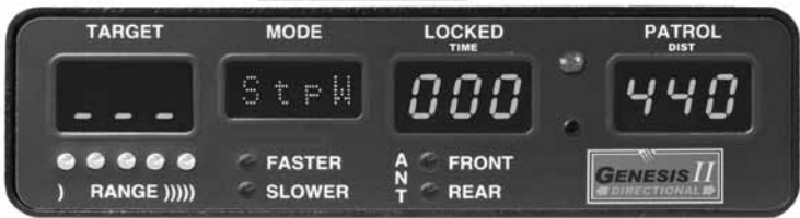
Figure 3-9a The Mode Window will display “StpW” whenever the Genesis-II Select Directional is operating in the Stopwatch Mode.
