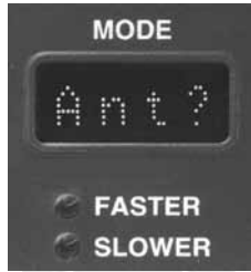
Figure 3.2a If no antenna is connected, Ant? displays.
