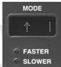
Figure 3.3f For a FRONT antenna selection, the Stationary Away Mode will show an arrow pointing up.
